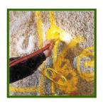
Sidewinder® is the winding configuration for NONEL LP series 5.4m. It has been specifically designed to reduce the occurrence of tangling of this shorter tube length on deployment. Each bundle holds 5 Sidewinder ® coils.
